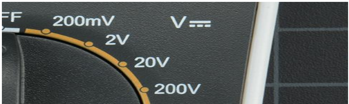
Figure 7: Use V with a straight line to measure DC Voltage
